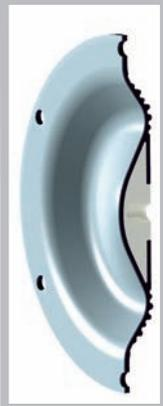
The surface of the ALMATEC diaphragms is smooth and not interrupted by any seals. Due to the integrated metal core, they do not require diaphragm disc which frequently give rise to leaks. ALMATEC diaphragms have always been designed from the "PTFE" point of view. Result: ALMATEC diaphragms have a large diameter and short stroke with low flexural load. ALMATEC diaphragms for the BIOCOR series are available in the materials EPDM (FDA) or PTFE/EPDM-composite.
