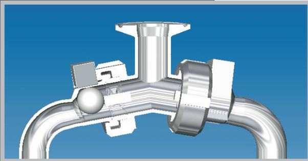
Always a demand for sterile applications: all housing parts of the BIOCOR pumps show no horizontal areas. Each pump of the B 20 and B 32 sizes comes with four ball lifting magnets, which can be attached to the pump housing from the outside at the location of the four ball valves. The ball valves are risen up magnetically out of their seats and the pump is drained entirely without having to be dismounted. There are no mechanical ball lifters with parts and seals in the wetted area.
